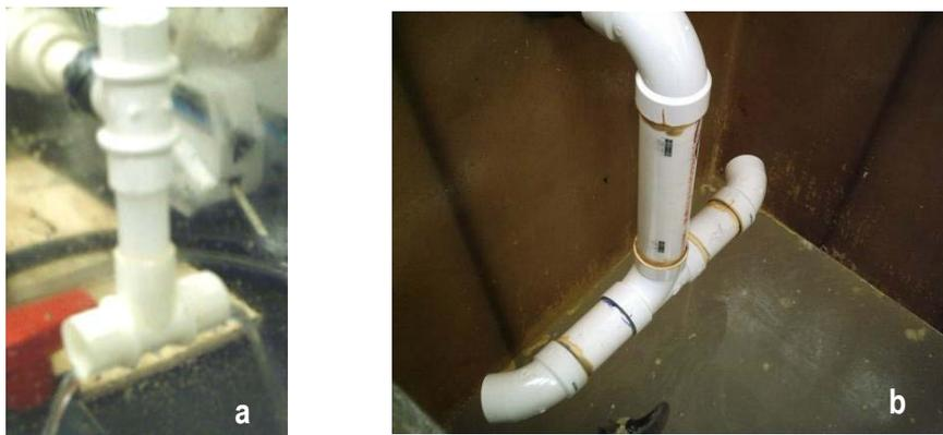
Figure 5-6. a) Bench Scale Distributive Inlet, b) Pilot/Field/CFD Distributive Inlet Configuration.
