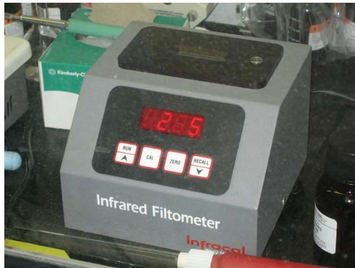
Figure 2-10. Infracal<sup>®</sup> Device Used for FOG Concentration Measurements.
