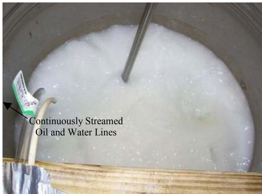
Figure 2-5. Oil/Water Mixing Drum.
