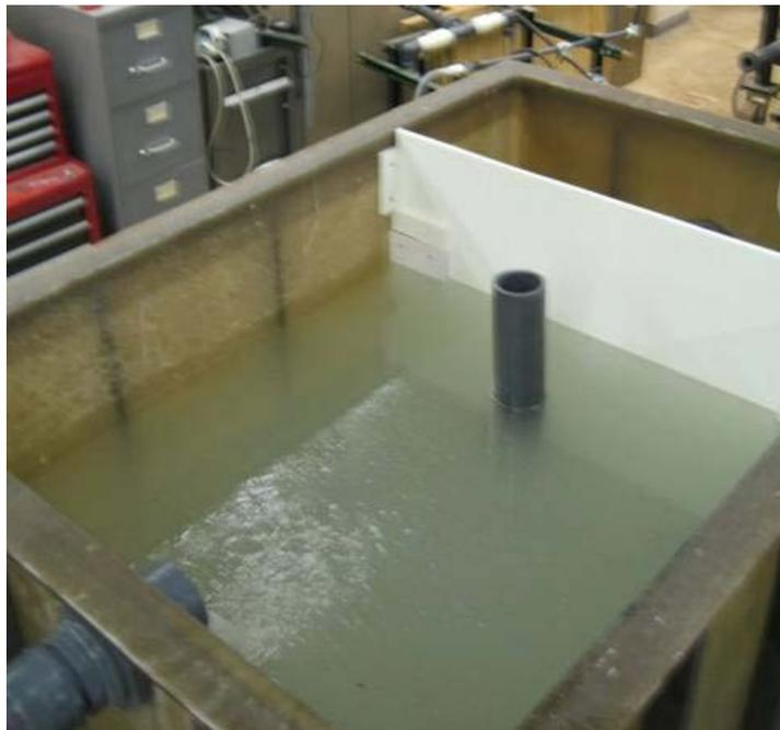
**Figure 2-3. Pilot Scale Grease Interceptor.**
