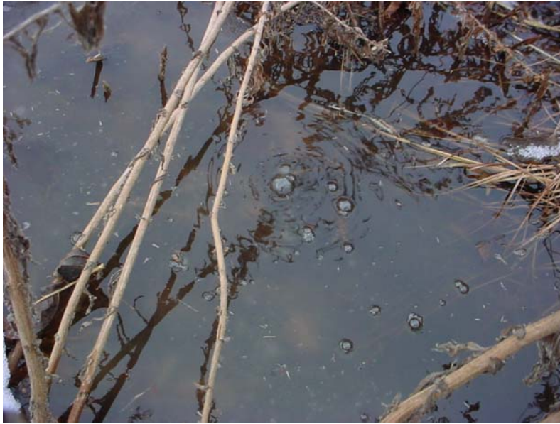
Figure 4-5. Photo of air escape from a mouse hole (biological permeability) during a DVD test with frost present.
