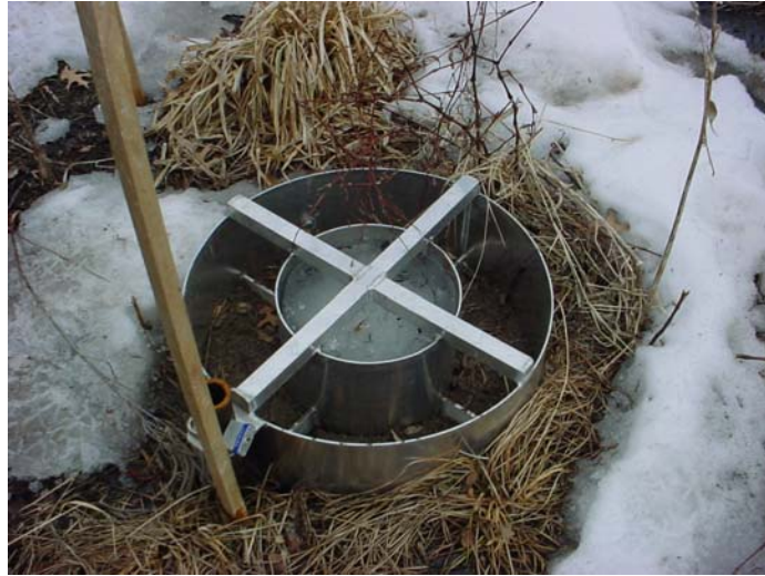
Figure 3-1. Photo of freezing associated with double-ring infiltrometer testing preventing use for study.
