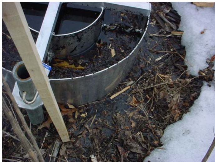
Figure 3-2. Photo of preferential thawing and flow around metal double-ring infiltrometers.
