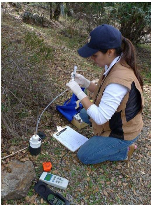
Figure 3-8. Sampling of Gases from the Venting System.
