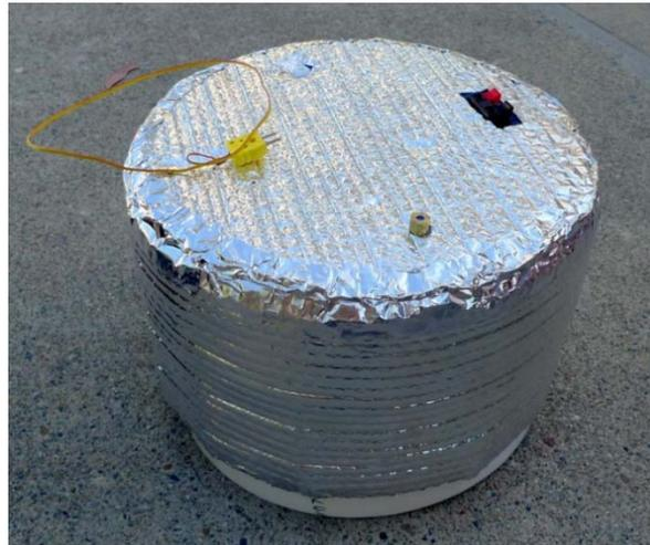
Figure 3-4. Flux Chamber Designed for Testing Gases from the Leach Field.
