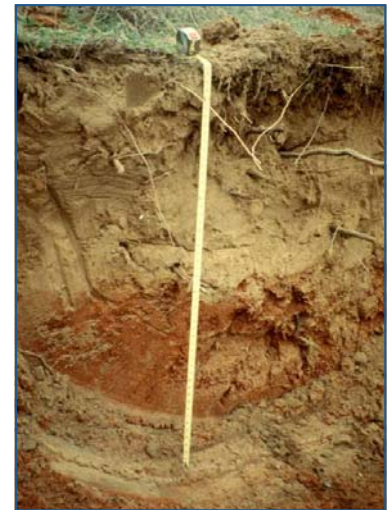
Gravity dispersal is most appropriate for sites with deep, well-drained soils.
