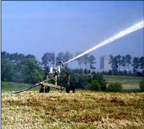
Traveling gun spray distribution components
