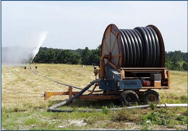
Traveling gun spray distribution components
