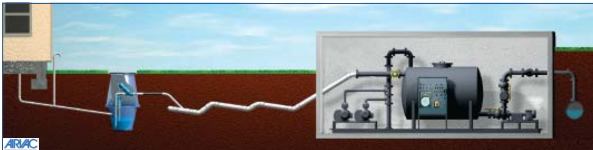
Pipes for vacuum sewers are installed in a saw-tooth or zigzag configuration to maintain a vacuum throughout the system.
