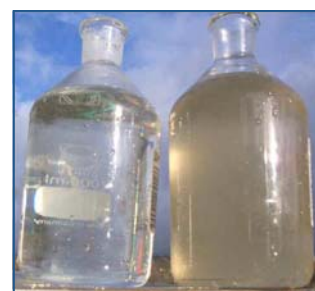
Effluent must be relatively clear in order for disinfection methods to be effective.
