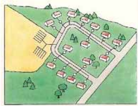
Figure 3-21 An Example Diagram of a Cluster Wastewater Treatment System
