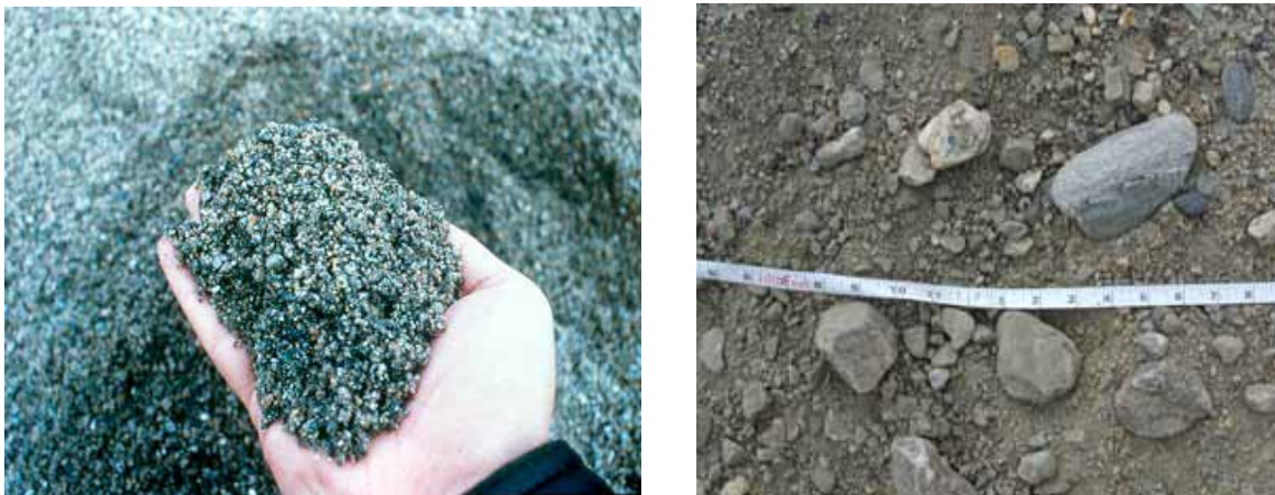
Figure 2-12 Sand Fill Used in the Wisconsin Mound (left) and Bank Run Gravel Used in Other Fill Systems (right)
